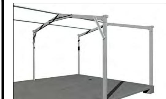
2A FIRST & SECOND PORTAL FRAME ASSEMBLY 1 REFER 2C FOR TEMPORARY BRACING LOCATION
