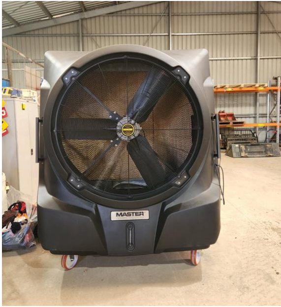
Photo: Mobile Evaporative air cooler
