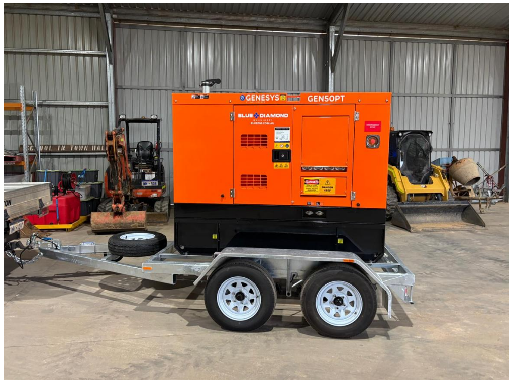
Photo: Mobile Generator – Recreation Centre
